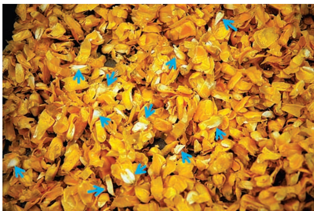
Figure 1. Solids recovered in treatment 4 (tail-end, wet-split degerm fermentation) before degerming. A few germ pieces are shown by arrows.
